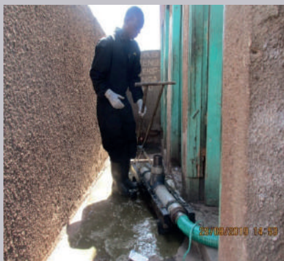
Gulper IV under development being tested
