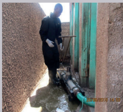
Gulper IV under development being tested
